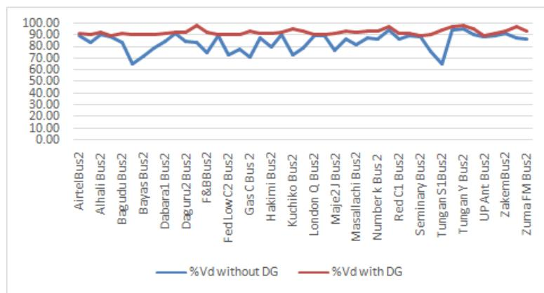
Figure 4.5: Voltage drops on Dikko Feeder With and Without DG.
