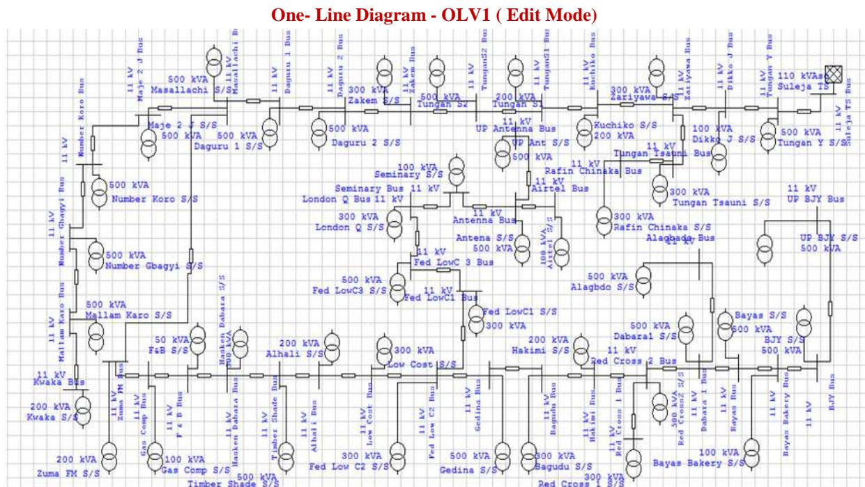
**Figure 3.7: Single Line Diagram of the Dikko Feeder Modeled in ETAP.**
