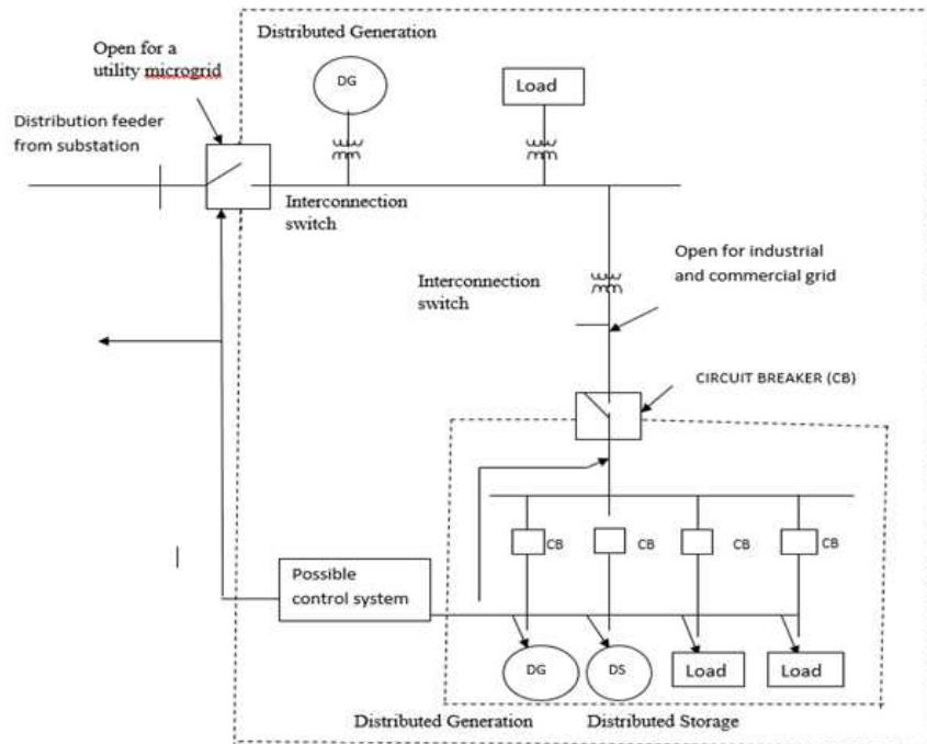
**Figure 2: Micro Grids and Components: [16].**
