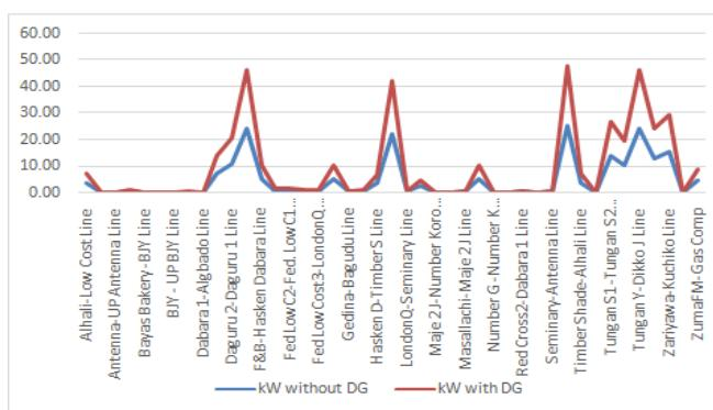
**Figure 4.3: Active Power Losses on Dikko Feeder With and Without DG.**
